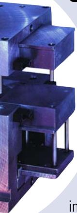
MUD H frame models offer simultaneous molding of two standard style companion insert molds. One insert mold can be run by installing the blank insert to block off one section of the frame. The mold ejector system can be tied to the frame master ejector plate with optional interlocking rails. H Series frames are well suited to both injection and transfer molding applications. A hot runner manifold can be added to combine the benefits of Quick-Change systems with hot runner molding.
